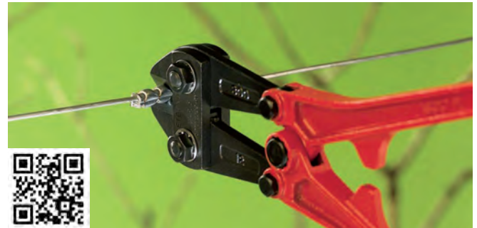
Crimping sleeve during crimping. Scan to view the video.
