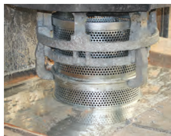
Parts dipped in the zinc bath.
