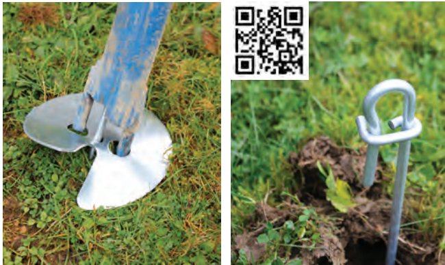
Helical anchoring disk with tubular driving tool. Scan to view the video.
