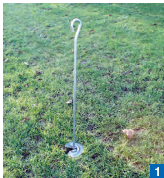
1 Screw the disk on the rod and start driving in the ground.
