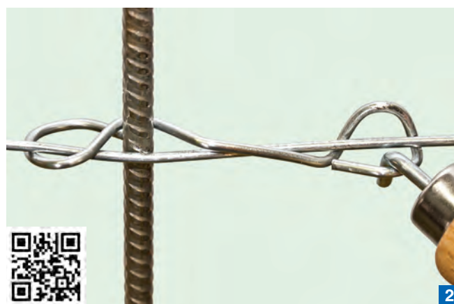
Place the hook of the handle in the folded loop of the clip and pass the loop under the wire. Scan to view the video.
